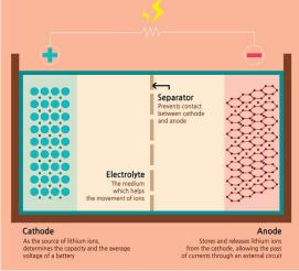
Figure 24 Components of a Li-ion Battery<sup>51</sup>
