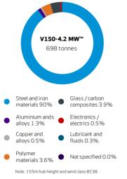
Figure 11 Materials required in a Vestas V150 4.2MW turbine<sup>26</sup>
